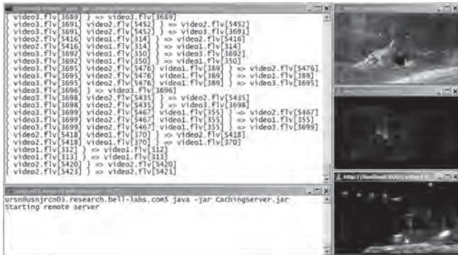
Fig. 7. Screenshot of video-streaming demo from [14]. The lower left window shows the server process. The upper left window shows the decoding process at a local cache. The three windows on the right show the reconstructed videos being played in real time.
