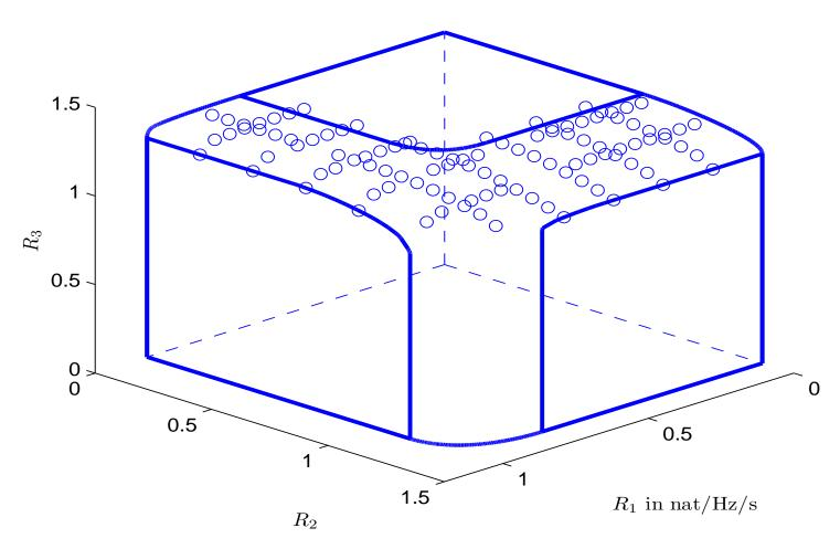
The convex hull of the SUD rate regions of a three-user MISO IC.
