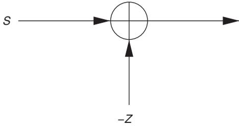
**Fig. 4** Equivalent additive-noise channel of a dithered lattice quantizer.  $\mathbf{Z}$  is independent of the input  $\mathbf{S}$ , and uniform over the fundamental region  $\mathcal{P}_0$  of  $\Lambda$ .
