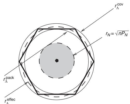
**Fig. 3** The fundamental Voronoi region and its packing radius, covering radius and effective radius (radius of the sphere having the same volume). Packing and covering efficiencies are measured by the corresponding ratios.
