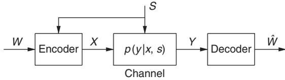
Fig. 6 A channel with side-information at the transmitter.
